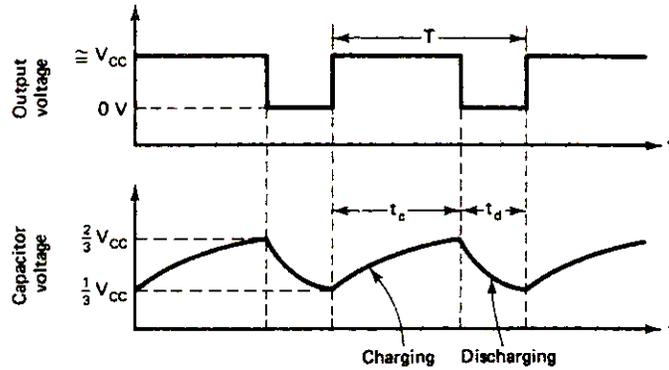
[Figure 4: Output voltage and capacitor voltage waveforms]
