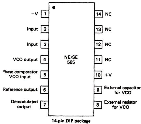
[Figure 8: Block diagram and pin diagram of phase locked loop]
