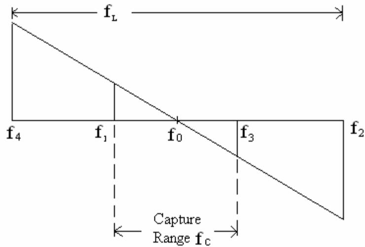
[Figure 10: Locking and Capture ranges of PLL]
