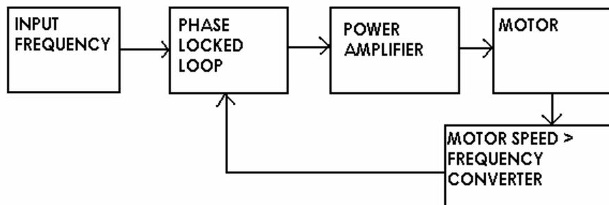
**[Figure 1: Basic blocks of the model]**
