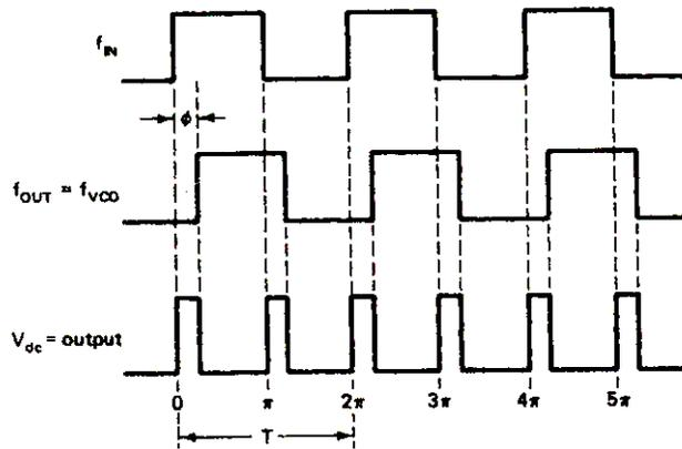
[Figure 7: Input and output waveforms]
