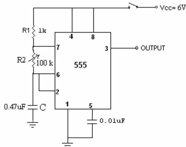
[Figure 3: Astable operation of 555]
