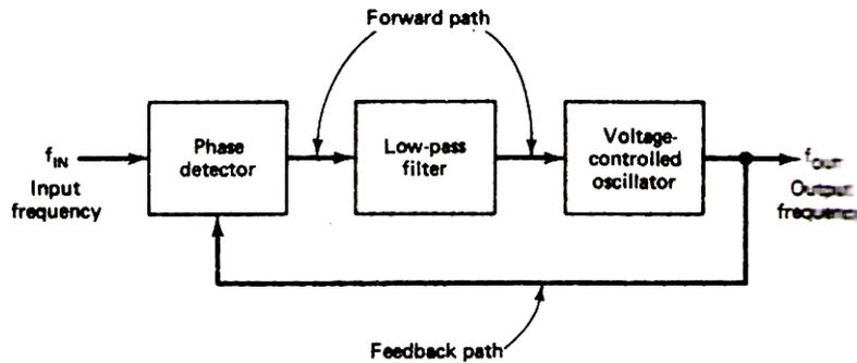
**[Figure 5: Idea of working of a phase-locked loop]**
