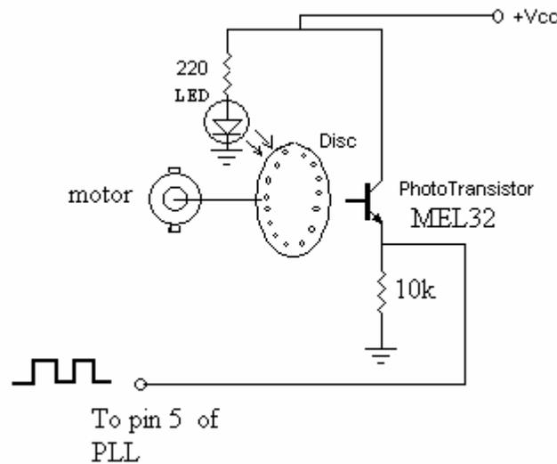
**[Figure 12: Speed to Frequency Converter]**
