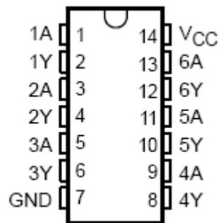
This 74HC04 device contains six independent inverters and performs the Boolean function  $Y = \overline{A}$  in positive logic.
