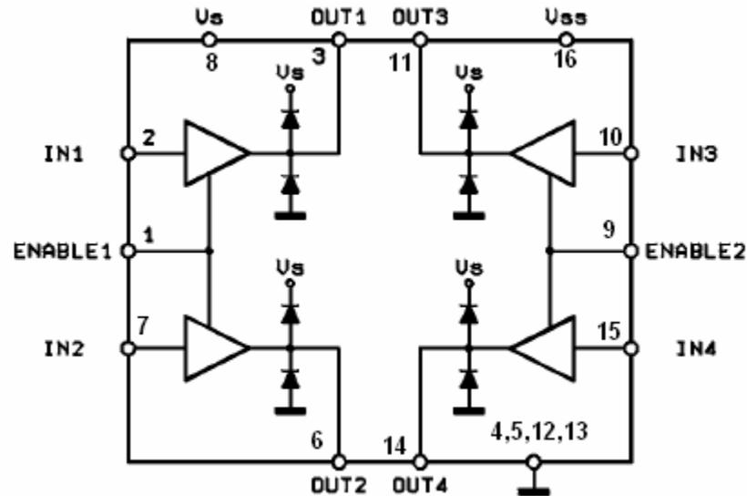
Figure 6.2 Block Diagram of L293D
